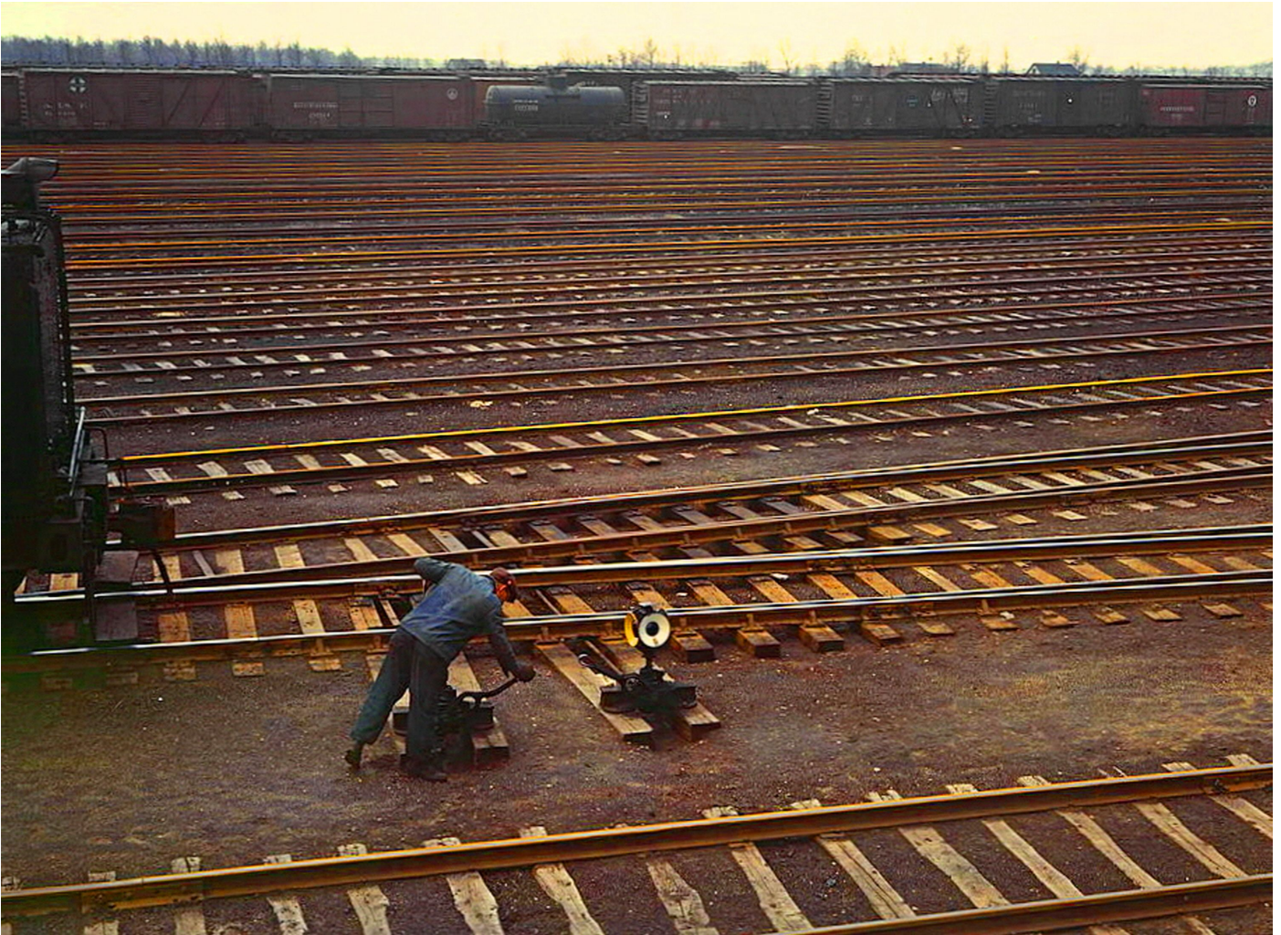
Delano, Jack (1914-) (photographer). Switchman throwing a switch at C & NW RR's Proviso yard, Chicago, Ill. U.S. Office of War Information (1943 April). No known restrictions on publication.
